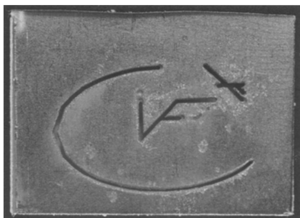
Fig. 10. Example of an acronym etched using a 219 \mu\text{m} nozzle; step length: 170 \mu\text{m} ; with laser assistance; average current density: 146 \text{kA m}^{-2} .
